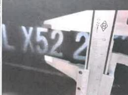
All pipes were marked with Manufacturer name, Standard, Size, Thickness, Length, Heat No., Serial No., API 5L
