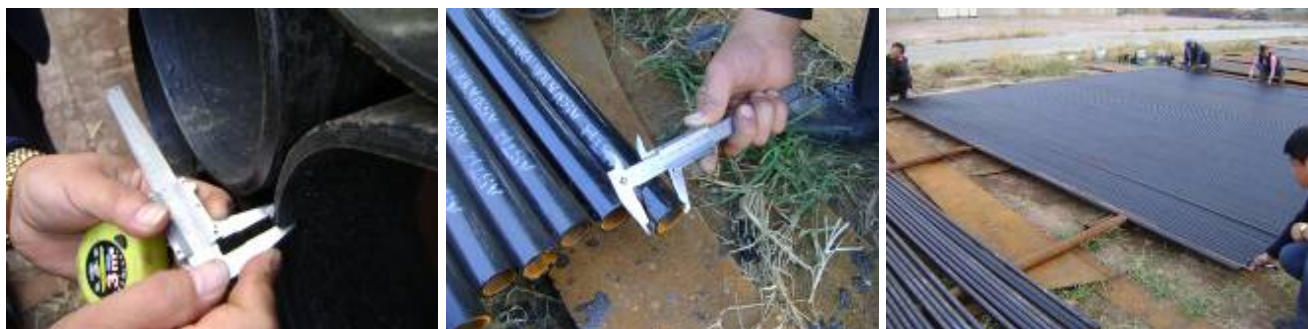
Outside diameter, wall thickness, length checking
