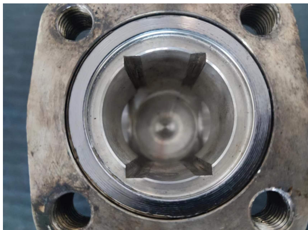
阀体-阀盖密封垫片 Body-Bonnet seal gasket
