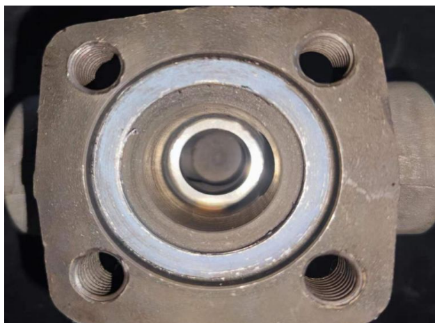
阀体-阀盖密封垫片 Body-Bonnet seal gasket
