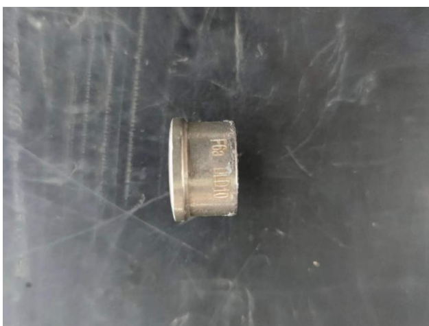
填料压套 Packing bushing
