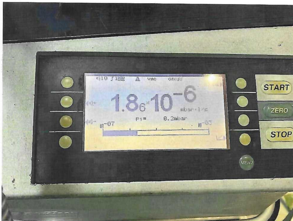
泄漏测量 leak measurement
