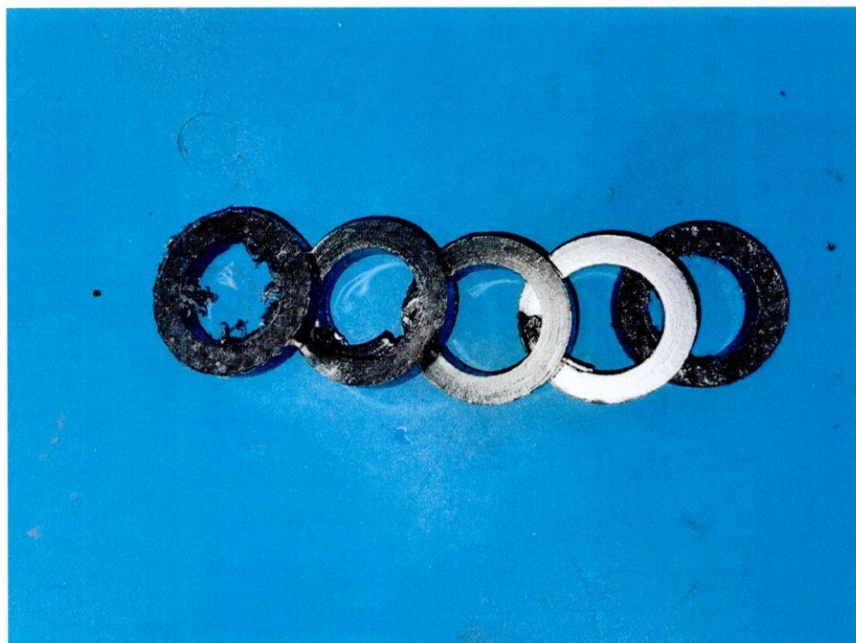
试验后的填料环 Packing rings after test
