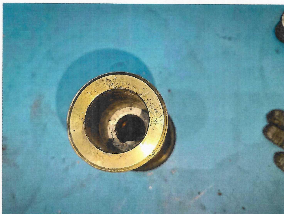
填料函 Packing sealing chamber
