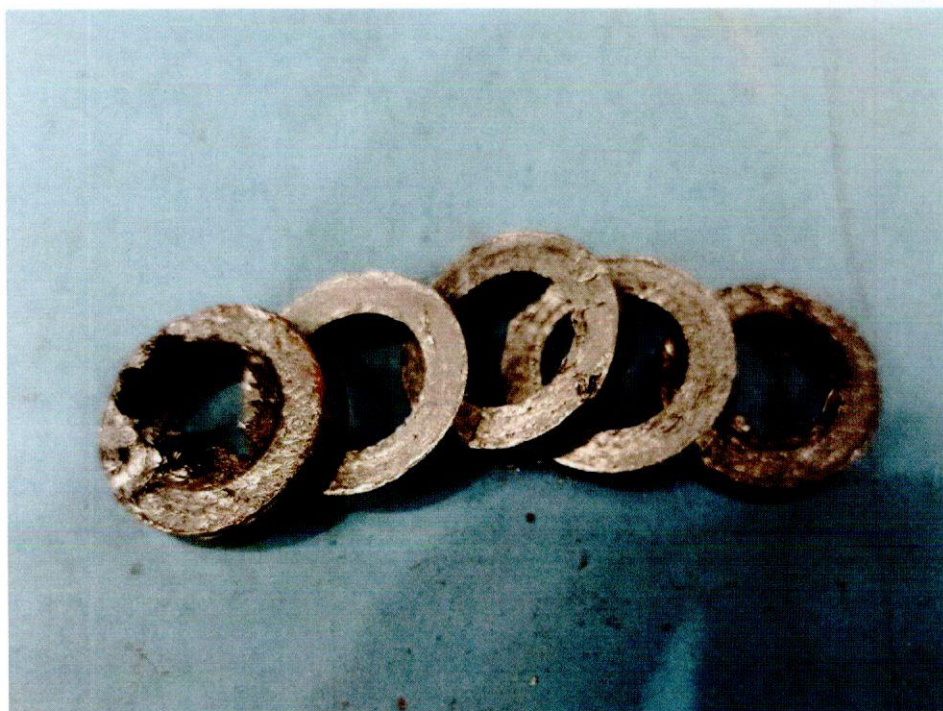
试验后的填料环 Packing rings after test
