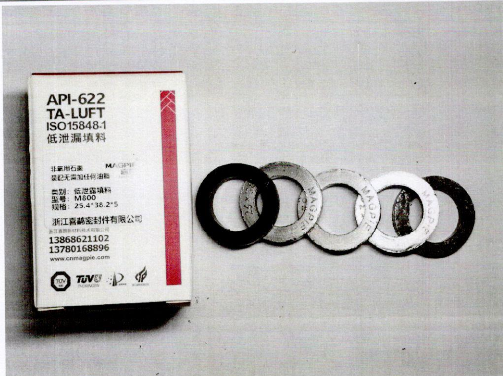
试验前的填料环 Packing rings before test
