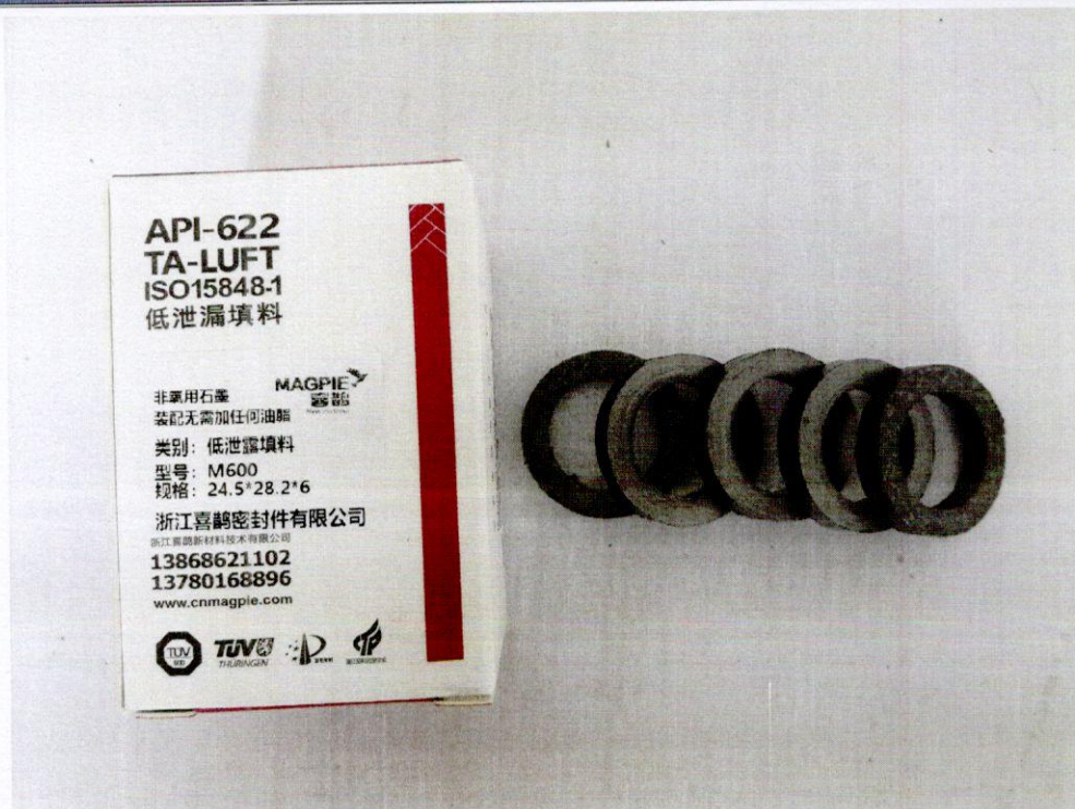
试验前的填料环 Packing rings before test
