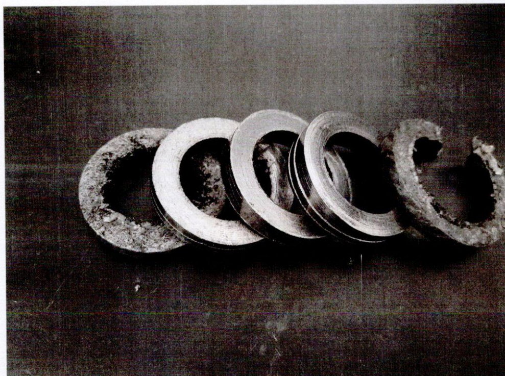
试验后的填料环 Packing rings after test
