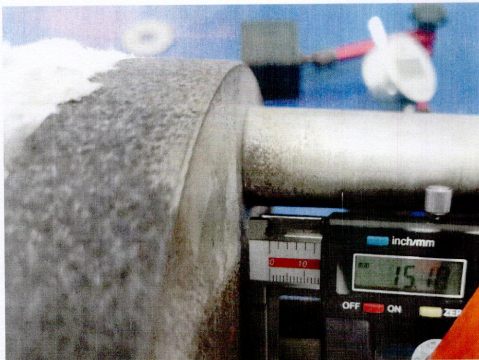
压缩高度测量 Packing Compression Measurement
