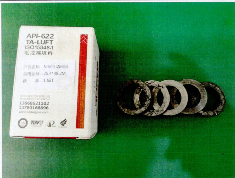
试验后的填料环 Packing rings after test
