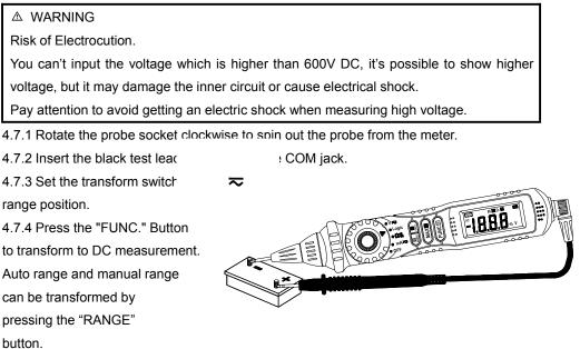
4.7.5 Connect the probe tip of the meter and probe tip of the test lead (or test clip) across the power source or be loaded on the two sides under measurement.
