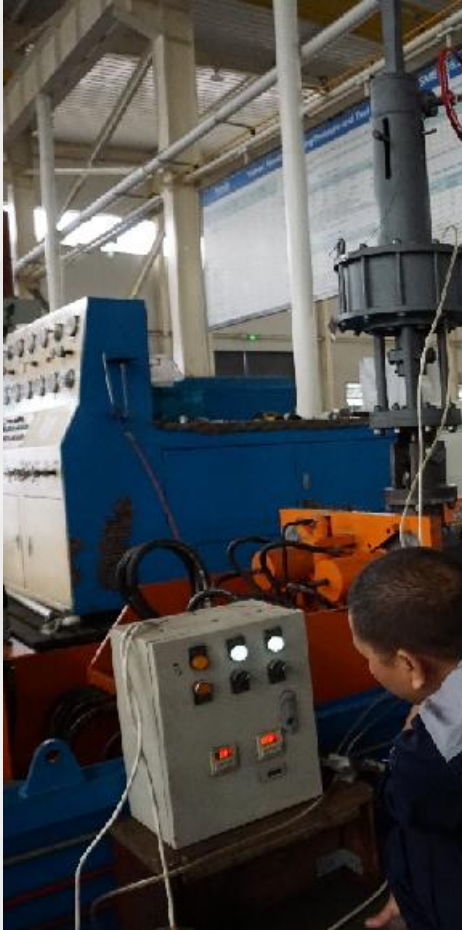
■ RISING STEM BALL VALVE 10,000 CYCLE TESTING
