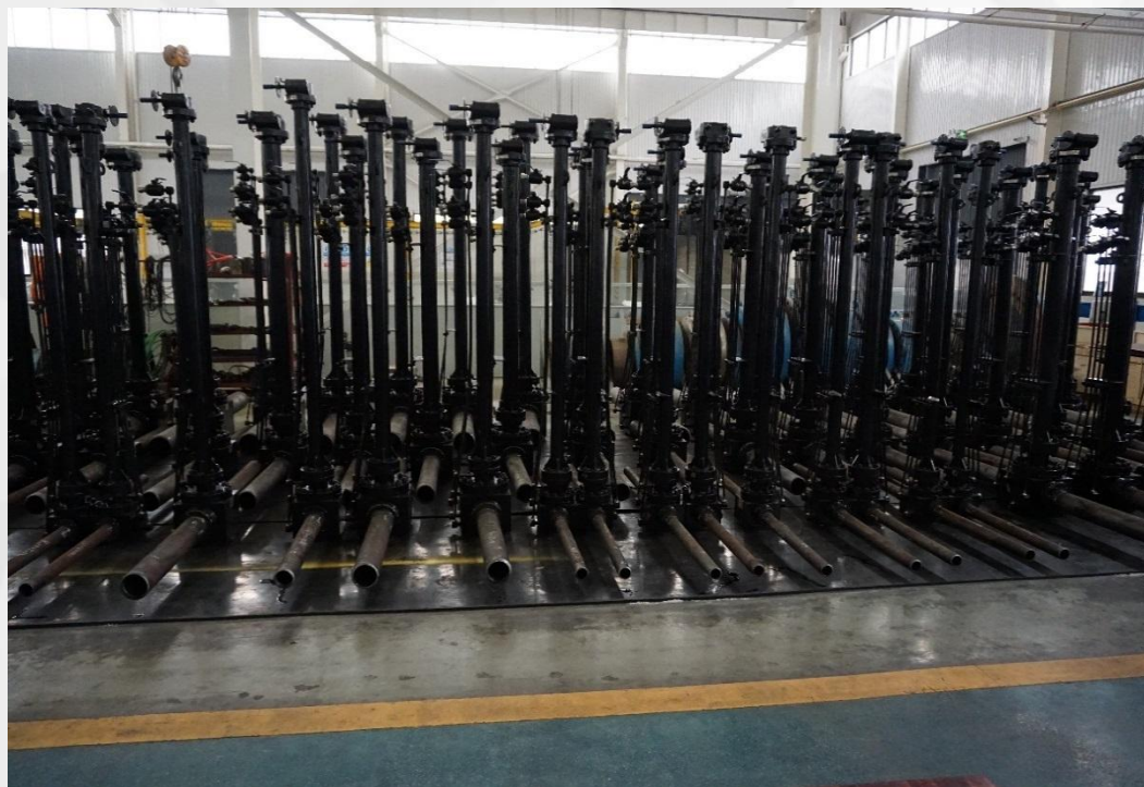
■ TOP ENTRY BALL VALVE WITH STEM EXTENSION LUKOIL
