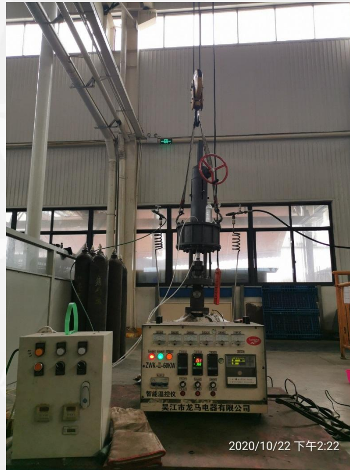
■ RISING STEM BALL VALVE HIGH TEMPERATURE TEST AT 362°C
