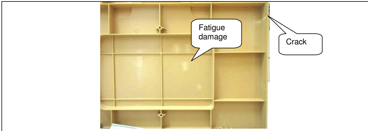
After test- Back of the plastic locker door
