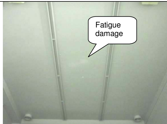
After test- Back of the plastic locker side face
