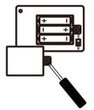
Open the back battery compartment on remote control panel with a screwdriver and install 4 AA batteries (not included). Close the lid and switch to "ON" with a power on signal.
