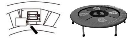
2. Open the back battery compartment on control panel with a screwdriver and install 4 AA batteries (not included). Close the lid and switch to "ON", it will play a power on signal.
