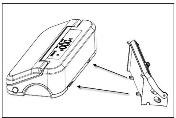
Follow the image above, put the buckle into the holes of the machine's body accordingly with enough strength.
