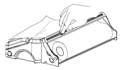
1. Put a bag roll into the roll holder, pull enough bag material to hold item to be vacuum packaged, plus 2 inches. Use the embedded cutter on the sealer to cut desired bag
