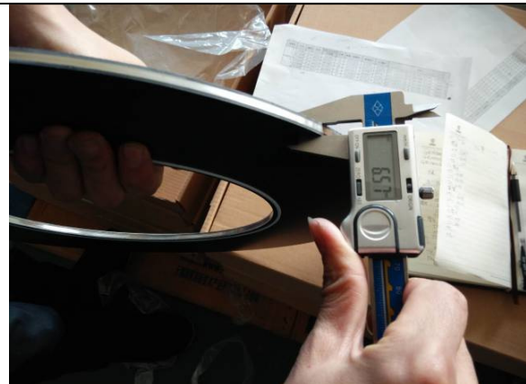
Thickness check for G10/316 gasket(THK1)
