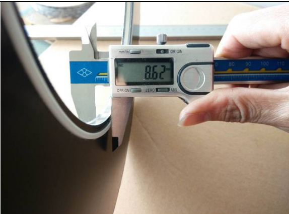
Thickness check for G10/316 gasket(THK2)
