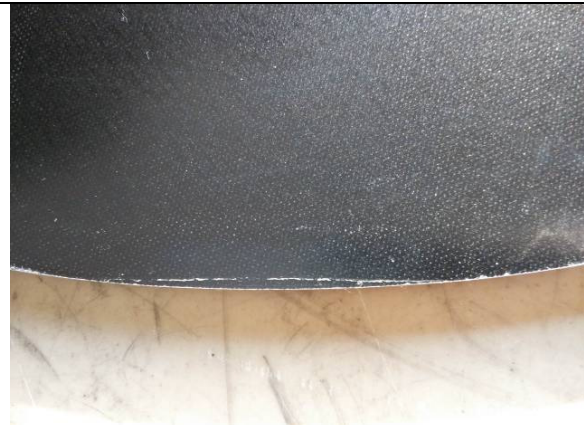
Slight scratch on gasket surface
