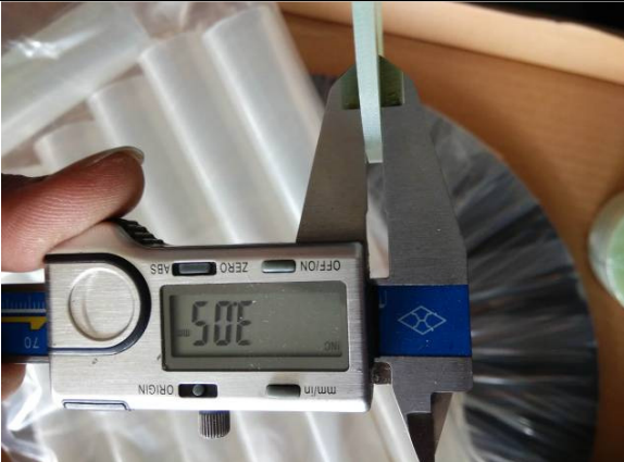
Thickness check for G10 retainer
