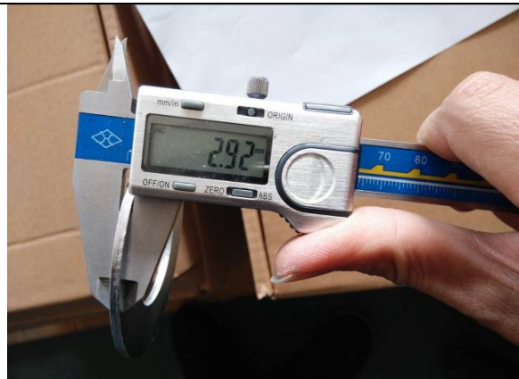
Thickness check for ZCP washer
