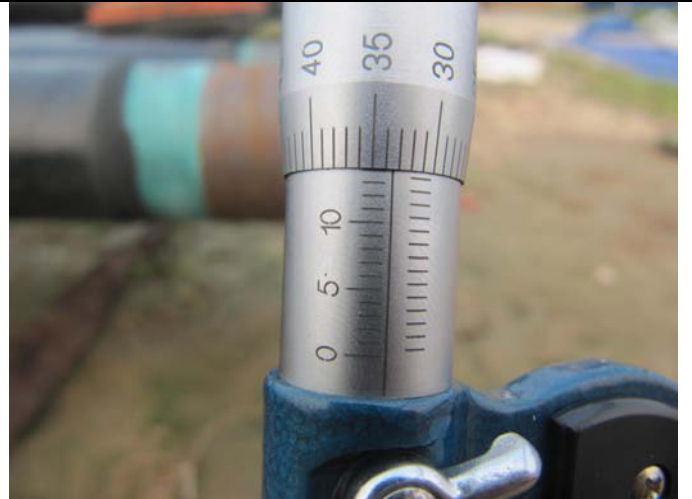
Pipe wall thickness check
