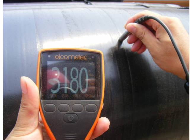
Total thickness of 3PE coating check
