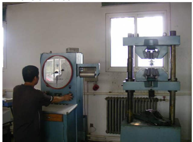
Witnessed tensile test
